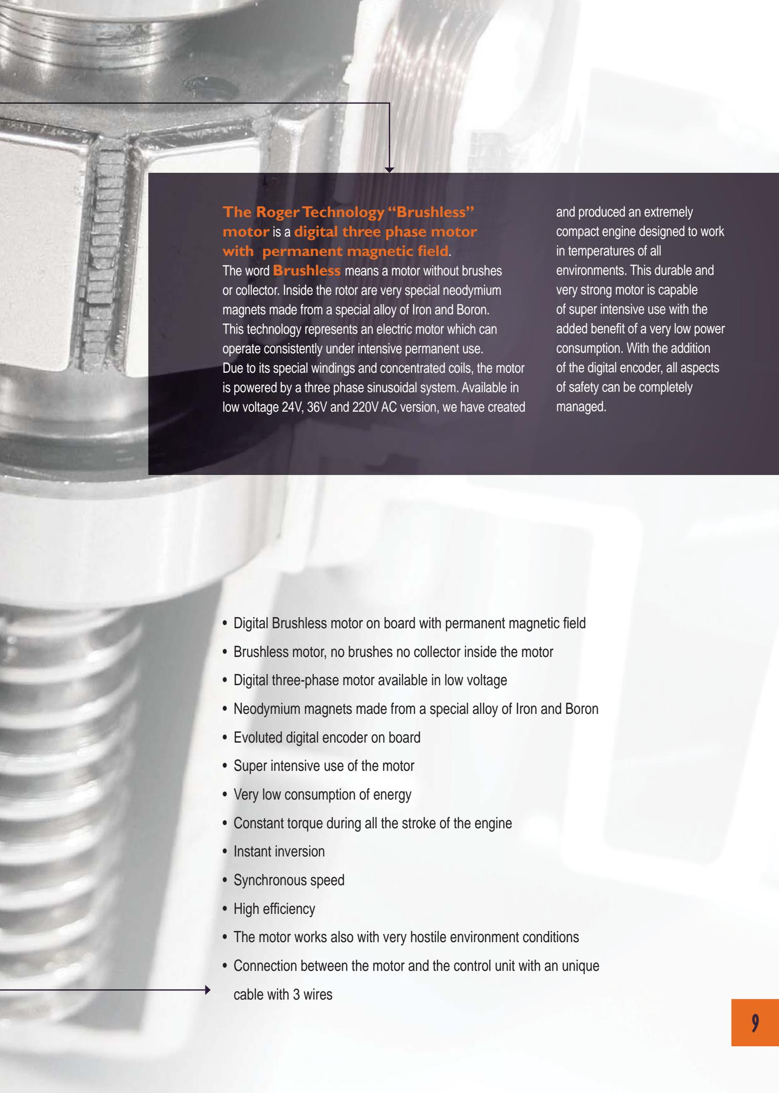
**The Roger Technology “Brushless” motor is a digital three phase motor with permanent magnetic field.**
